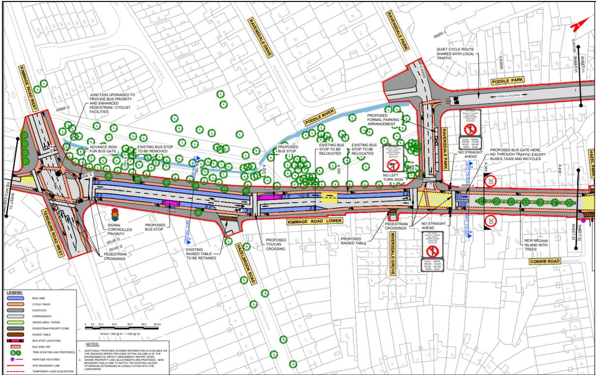
Figure 2-1-1: Extract from General Arrangement Drawings (Sheet 1)
