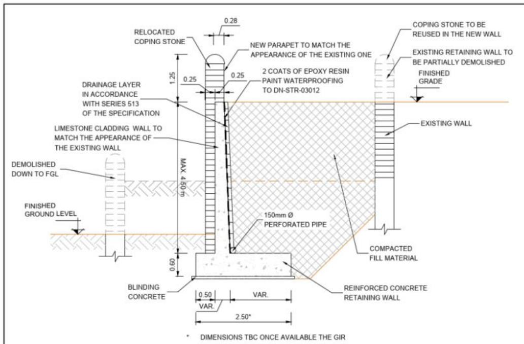
**Figure 8.12: Kimmage 03 – Typical Cross Section of Retaining Wall**
