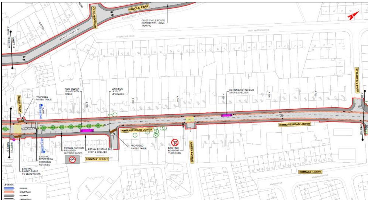
Figure 2-1-2: Extract from General Arrangement Drawings (Sheet 2)
