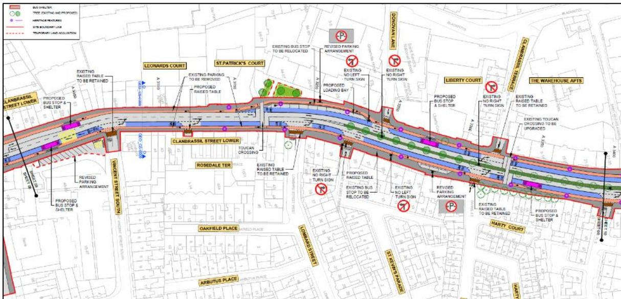
Figure 2-3-2: Extract from General Arrangement Drawings (Sheet 9)
