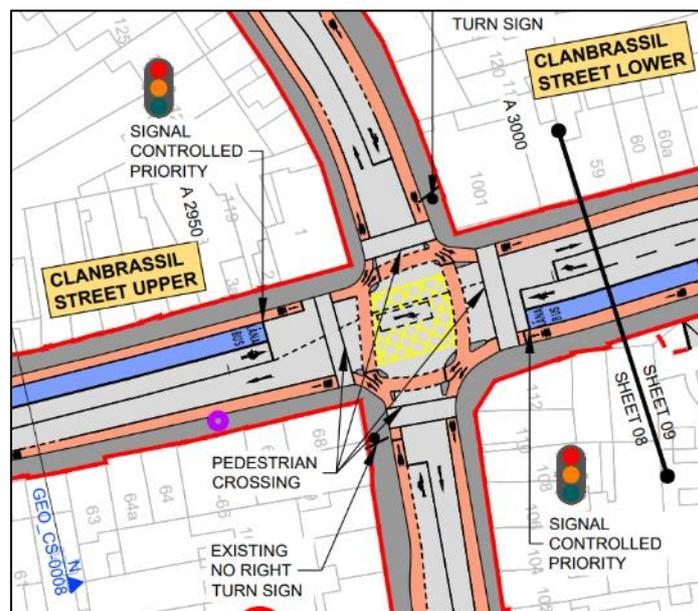
**Figure 2-9-5: Proposed Scheme Layout at Leonard’s Corner Junction**
