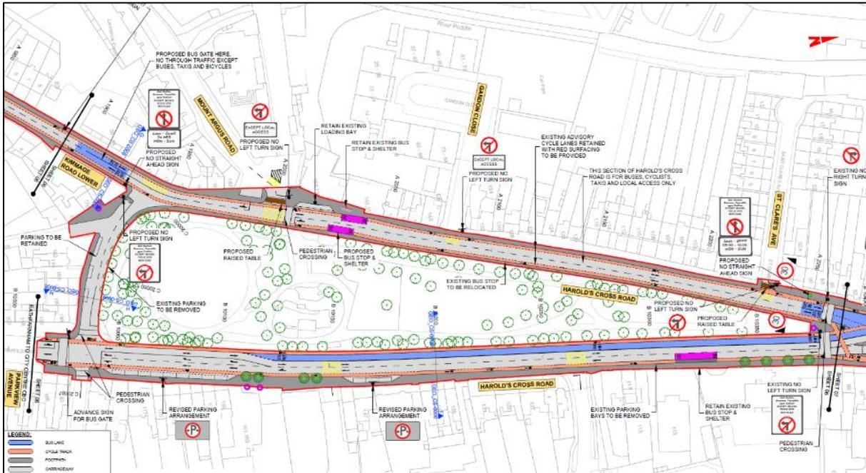
Figure 2-1-6: Extract from General Arrangement Drawings (Sheet 6)
