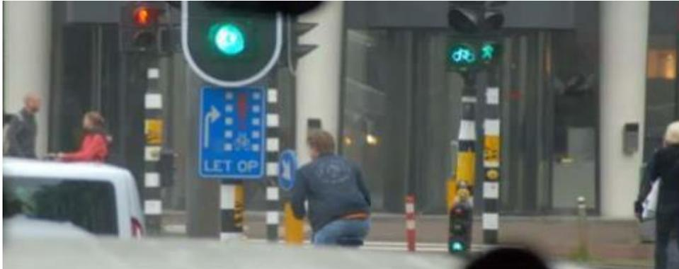
**Figure 2.4.2 Example from the Netherlands of traffic signals + give way signage controlling turning traffic and cyclists (Source: Dutch Design Guide Ontwerpwijzer Fietsverkeer)**
