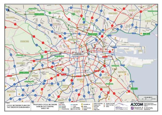
Figure 4-4 - GDA Cycle Network Plan for Central Dublin
