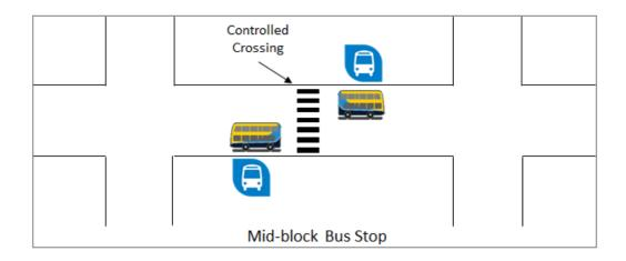
Figure 5.10 Mid-block bus stop optimum layout.
