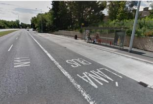
**Figure 1.5** Stillorgan QBC with high bus flows and no bus laybys resulted in bus bunching/ platooning; bus lay-by's provided at key locations to allow express buses to pass slower buses. (Source: Google Maps)
