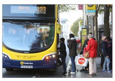
**Figure 5.12** Having buses flush with the bus stop is important to allow the ramp to lower correctly, but also to speed up the boarding and alighting of all passengers as gaps slow this down.
