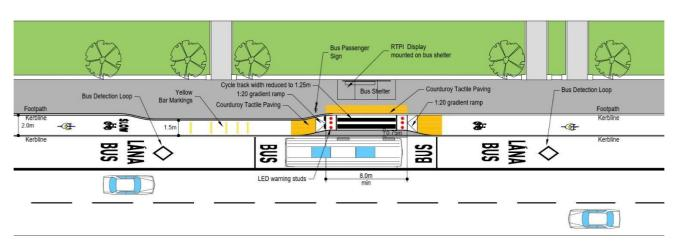
Figure 5.4 Shared Bus Stop Landing Zone Arrangement (Bus Connects Design Guideline).
