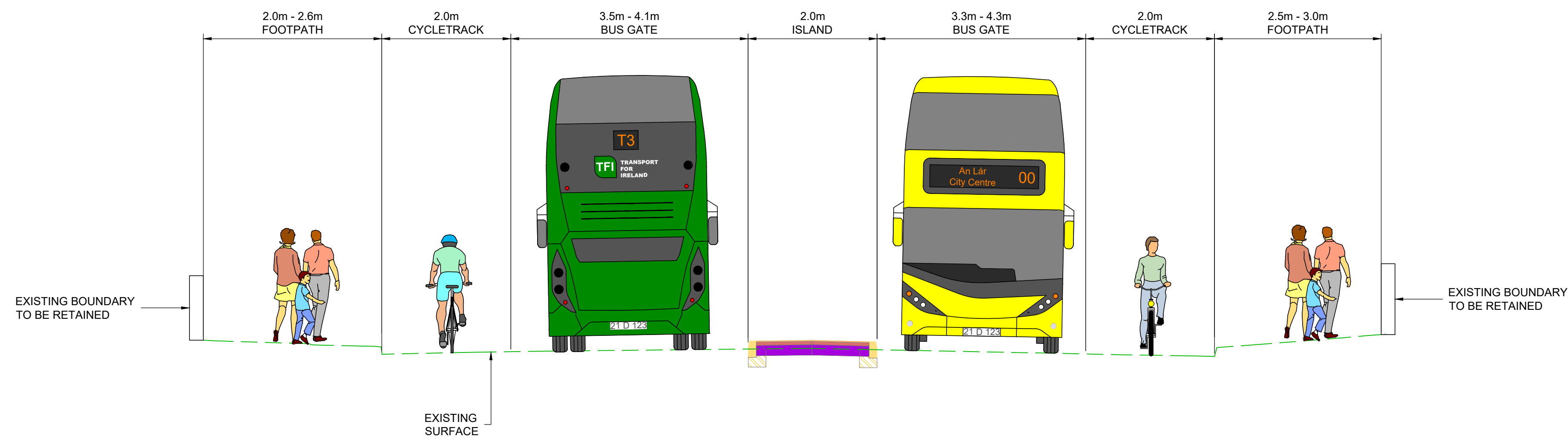
TYPICAL CROSS SECTION B-B KIMMAGE ROAD LOWER LOCATED ON GA SHEET 01 DRAWING REF: BCIDD-ROT-GEO_GA-0011_XX_00-DR-CR-0001
