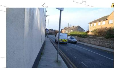
CHECK POSITION OF SIGNAL POLES FOR NOT REDUCING FOOTPATH WIDTH. THE MINIMUM DISTANCES WHEN OBSTACLES CANNOT BE REMOVED SHOULD BE 1500MM. AND 1200 IN SOME POINTS
