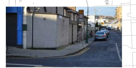
UNCONTROLLED CROSSING WITH NO TACTILE PAVING AND DISHED KERB. ACCESSIBILITY MEASURES FOR THIS TYPE OF CROSSING SHOULD BE PROVIDED. A DISHED KERB AND BUFF" OR GREY TACTILE PAVING SHOULD BE CONSIDERED (FOR AN IN LINE CROSSING). DEPTH OF 1.2 M, GRADIENT 1:12 MAX.
