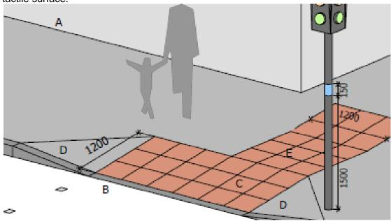
Figure 16. Controlled Crossing. In Direct Line of Travel
