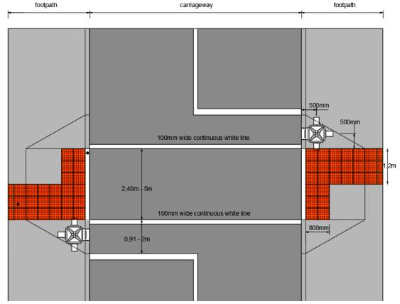
Figure 15. Controlled Crossing. Not in Direct Line of Travel
