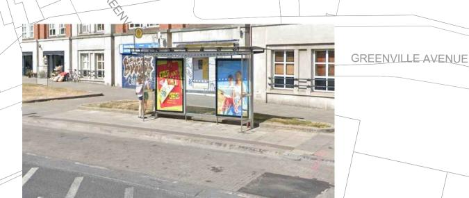
AN ISLAND BUS OPTION IS PROPOSED IN THE DESIGN PROJECT. IT SHOULD BE CONSIDERED FOR AVOID THE PEDESTRIAN/CYCLIST CONFLICT, WITH AN ON DEMAND SIGNALISED PEDESTRIAN CROSSING (TACTILE PAVING; PUSH BUTTON, LED WARNING STUDS) AND A SECONDARY UNCONTROLLED CROSSING ON THE DOWNSTREAM OF THE ISLAND. DESIGNERS SHOULD NARROW THE CYCLE TRACK TO LESS THAN 2.0 M.
