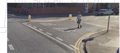
UNCONTROLLED CROSSING WITH NO TACTILE PAVING AND DISHED KERB. ACCESSIBILITY MEASURES FOR THIS TYPE OF CROSSING SHOULD BE PROVIDED. A DISHED KERB AND BUFF" OR GREY TACTILE PAVING SHOULD BE CONSIDERED (FOR AN IN LINE CROSSING). DEPTH OF 1.2 M, GRADIENT 1:12 MAX. LEVEL DIFFERENCE OF DISHED KERB: 6MM IF THE CENTRAL ISLAND IS INTENDED AS AN AREA TO WAIT THEN TACTILE PAVING TO BE ALSO PROVIDED INSIDE. OPTIMUM TIME OF CROSSING SHOULD BE CHECKED.
