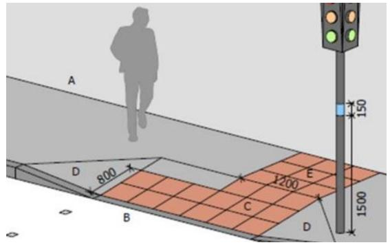
Figure 17. Controlled Crossing. Not in Direct Line of Travel
