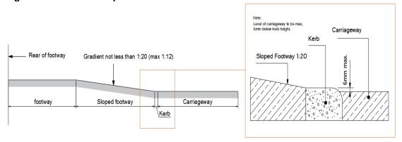
Figure 8. Dished Kerb Section Detail
