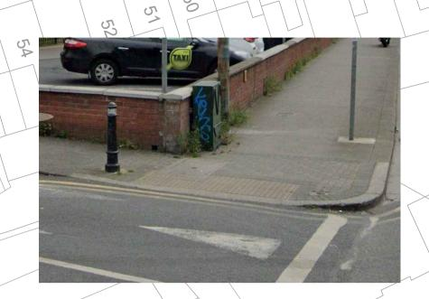
IN THE UNCONTROLLED CROSSING POINT.IF THE CROSSING IS IN LINE. THE "BUFF" OR GREY TACTILE PAVING SHOULD HAVE 1200 MM WITDH . (3 SLABS). ANOTHER ONE ROW OF SLABS SHOULD BE DISPOSED.
