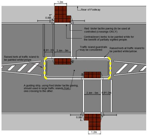
Figure 18. Controlled Crossing. Staggered Signalized Crossing
