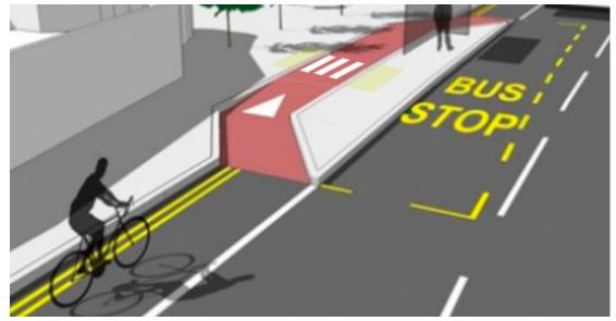
Example of a bus stop bypass solution
