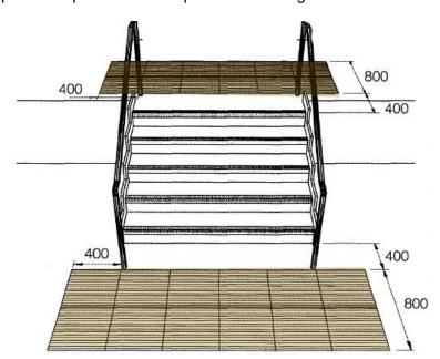
Layout of corduroy hazard warning surface at the top& bottom of a flight of stairs
