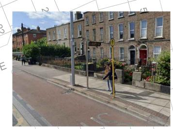
REDUCED LENGTH OF THE PICK UP POINT IN THE BUS STOP. IT CAN BE A HAZARD IN THE ACCESS FOR PEOPLE WITH MOBILITY MPAIRMENT. AN APPROPRIATE DISTANCE BETWEEN SIGNALS POLES SHOULD BE PROVIDED.
