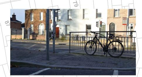
CONTROLLED CROSSING WITH A HIGH UPSTAND. THE LEVEL DIFFERENCE IN THE DISHED KERB SHOULD NOT BE HIGHER THAN 6MM. FOR AVOIDING HAZARD FOR WHEELCHAIR USERS AND PEOPLE WITH MOBILITY IMPAIRMENTS.
