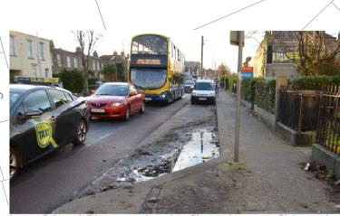
CHECK THE DRAINAGE SYSTEM IN CAR PARKING. INADEQUATE CROSS FALL CAN CAUSE ACCUMULATION OF WATER AND MAKE SURFACES TO BE SLIPPERY.
