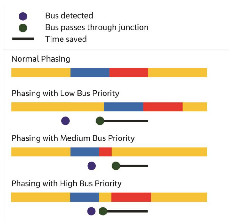
Diagram 7.2 Principles for high, medium and low bus priority
