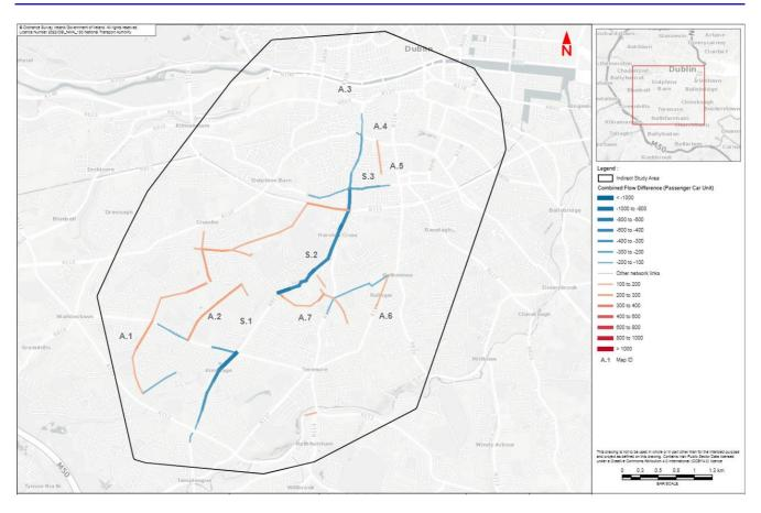
Diagram 6.19 Flow Difference on Road Links (Do Minimum vs. Do Something), AM Peak Hour, Opening Year (2028)
