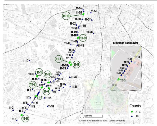
Diagram 5.1: Automatic Turning Counts (ATCs) and JTC Traffic Counts Locations
