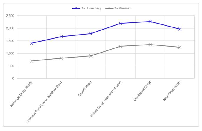
Diagram 6.7 2028 AM Peak Hour Passenger Volume Along Proposed Scheme (inbound direction)
