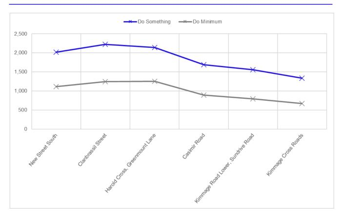
Diagram 6.10 2043 PM Peak Hour Passenger Volume Along Proposed Scheme (outbound direction)
