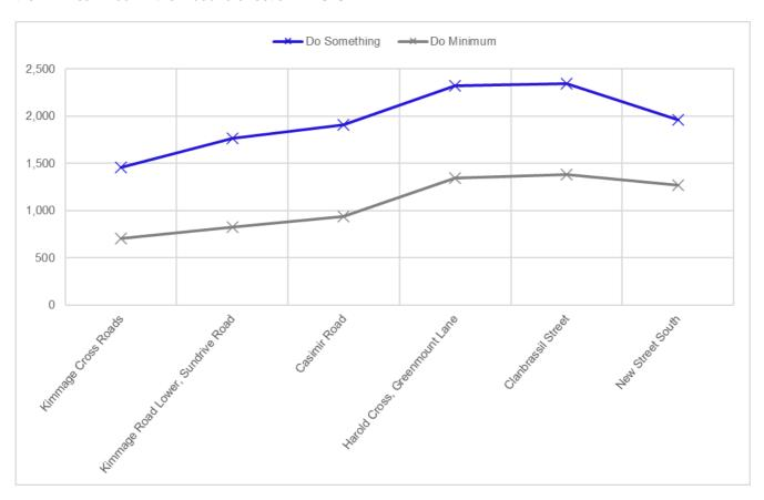
Diagram 6.8 2043 AM Peak Hour Passenger Volume Along Proposed Scheme (inbound direction)
