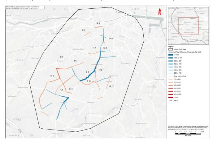
Diagram 6.20 Flow Difference on Road Links (Do Minimum vs. Do Something), PM Peak Hour, Opening Year (2028)
